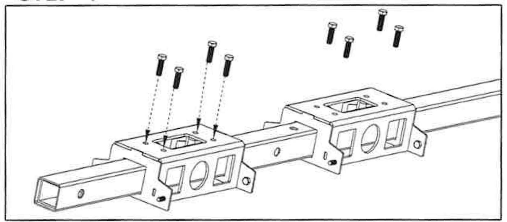
Slide rail brackets onto main holding tube and adjust according to desired length. Tighten the four 3/8"x 3/4" bolts for each bracket to lock position of rail brackets. This setting can be readjusted at a later time.
