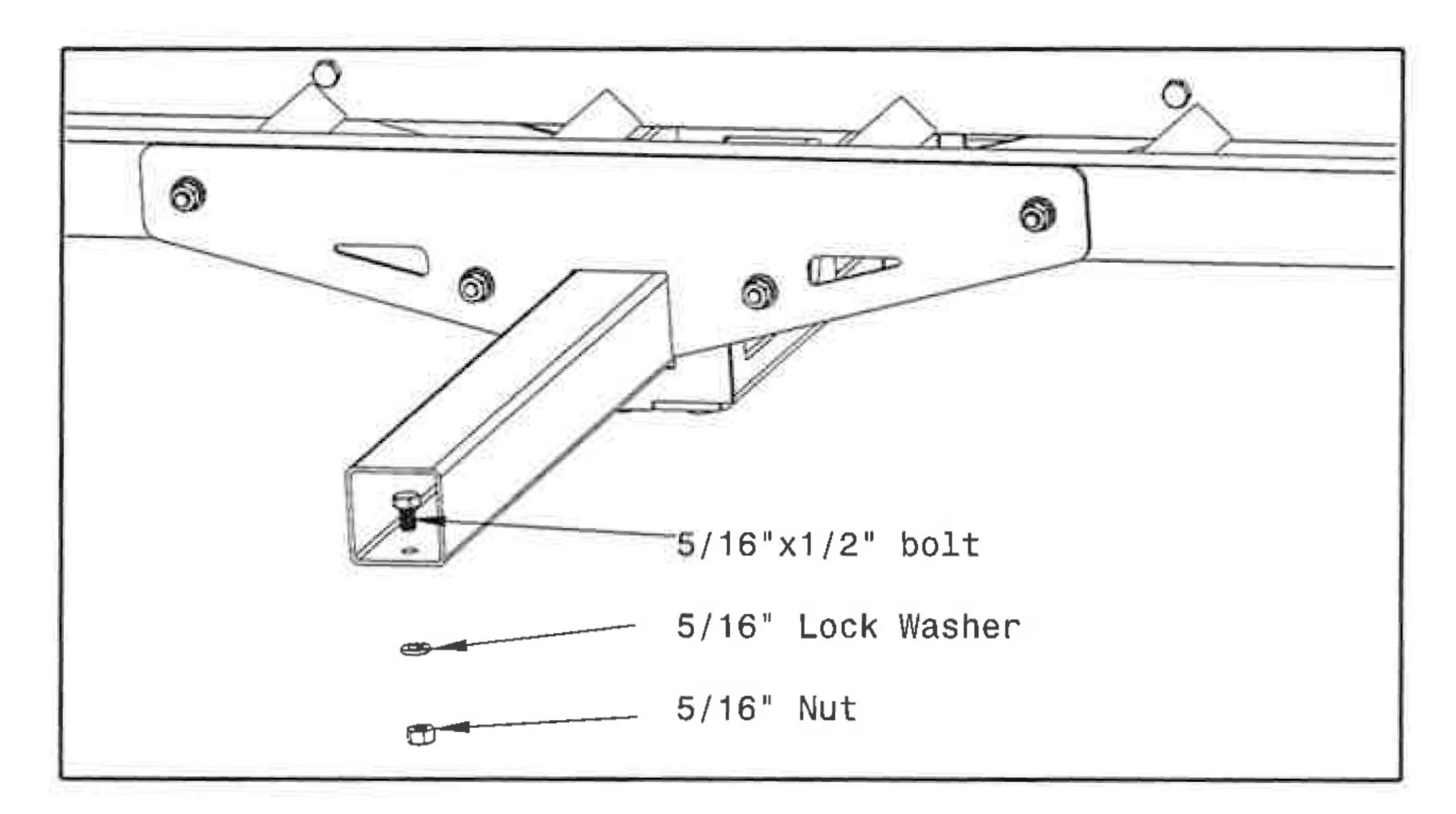
As a final safety precaution, bolt in and tighten a 5/16"x1/2" bolt at the end of the main holding tube, together with the 5/16" lock washer and nut.
