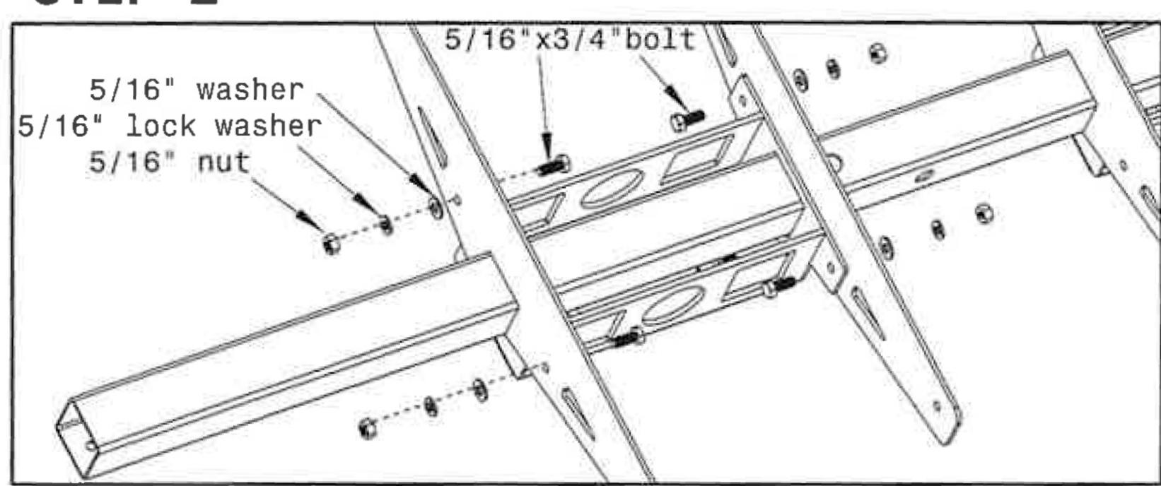
Attach the side rail brackets to the sides of the center rail bracket. Bolt them together using the 5/16"x3/4" bolts, 5/16" washers, lock washers and nuts. Do not tighten the bolts just yet. Leave them loose until the rails are installed.
