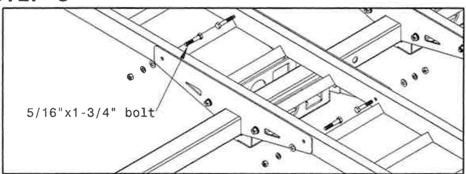
Now insert the 2 main rails into the previously assembled brackets. Bolt the rails to the brackets using 5/16"x1-3/4" bolts, 5/16" washers, lock washers and nuts. Now tighten all 5/16" bolts, including the ones left loose previously.
