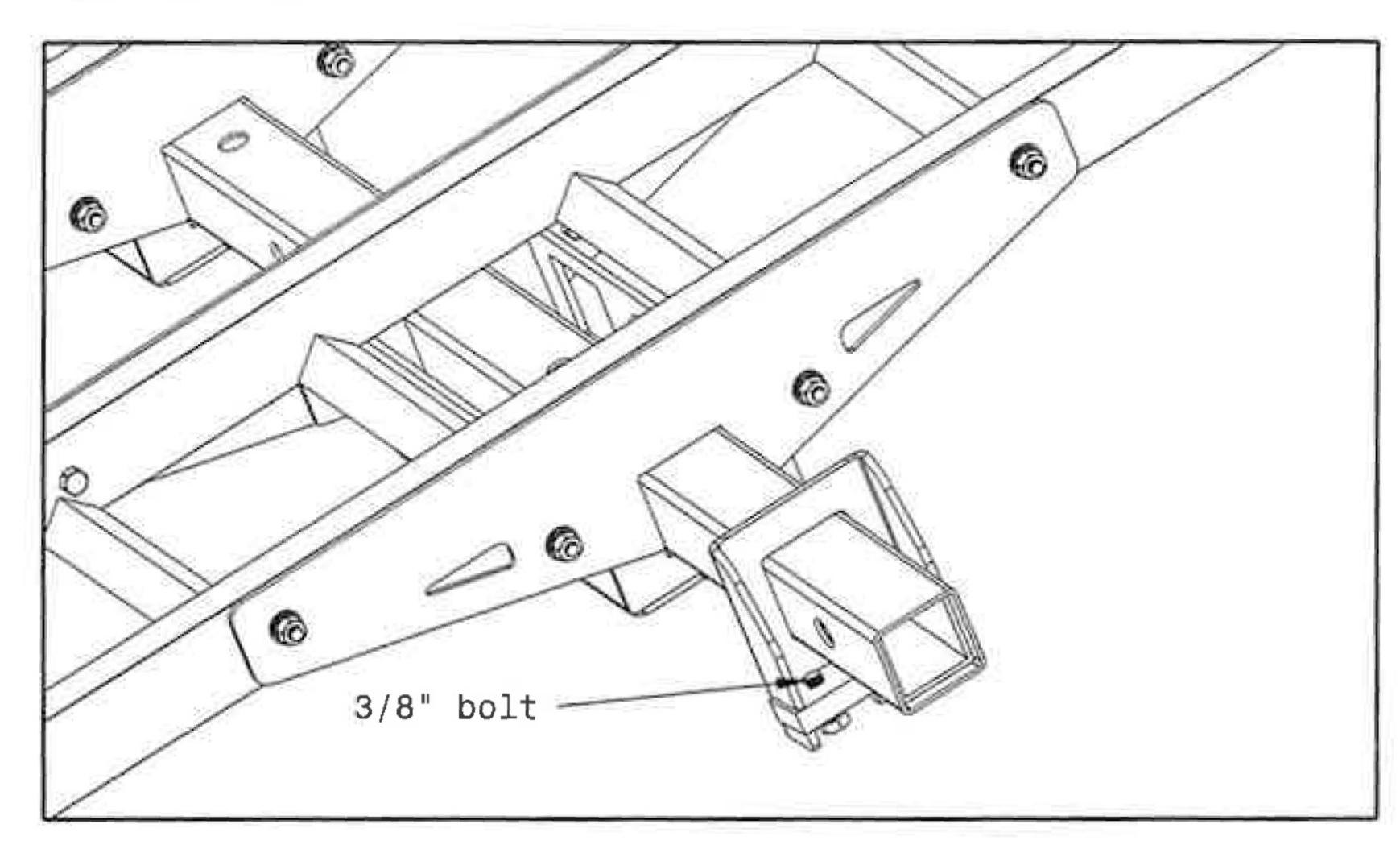
Insert the Anti-tilt bracket onto the Main Tube and insert the carrier into your hitch receiver.
